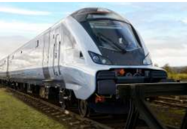
Chiltern Mk. 5 driving trailer (unpowered). The motive power goes on the other end.
